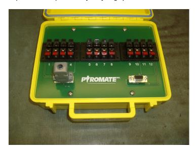
Firing module with shunt device inserted into firing cable input connector.
