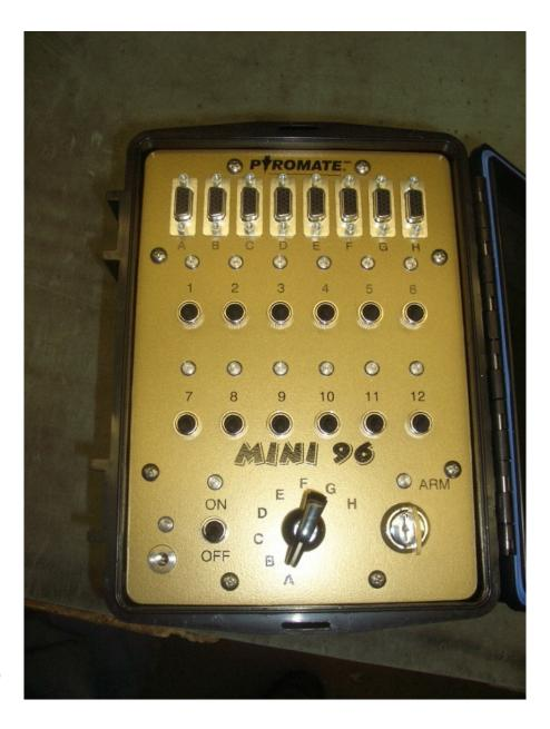
The Pyromate Mini 96 pyrotechnic firing system provides the ability to individually apply an activating voltage to 1 to 12 separate circuits. The 24 volt power source is internal to the control panel and is recharged thru the charge jack using a 12 VDC external power supply.
